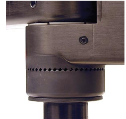
Figure 11 - INCORRECT: Rosette joints not aligned
