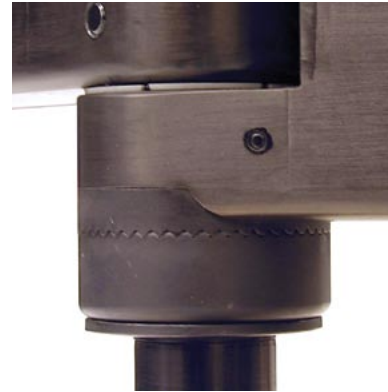
Figure 10 - CORRECT: Rosette joints nested properly
